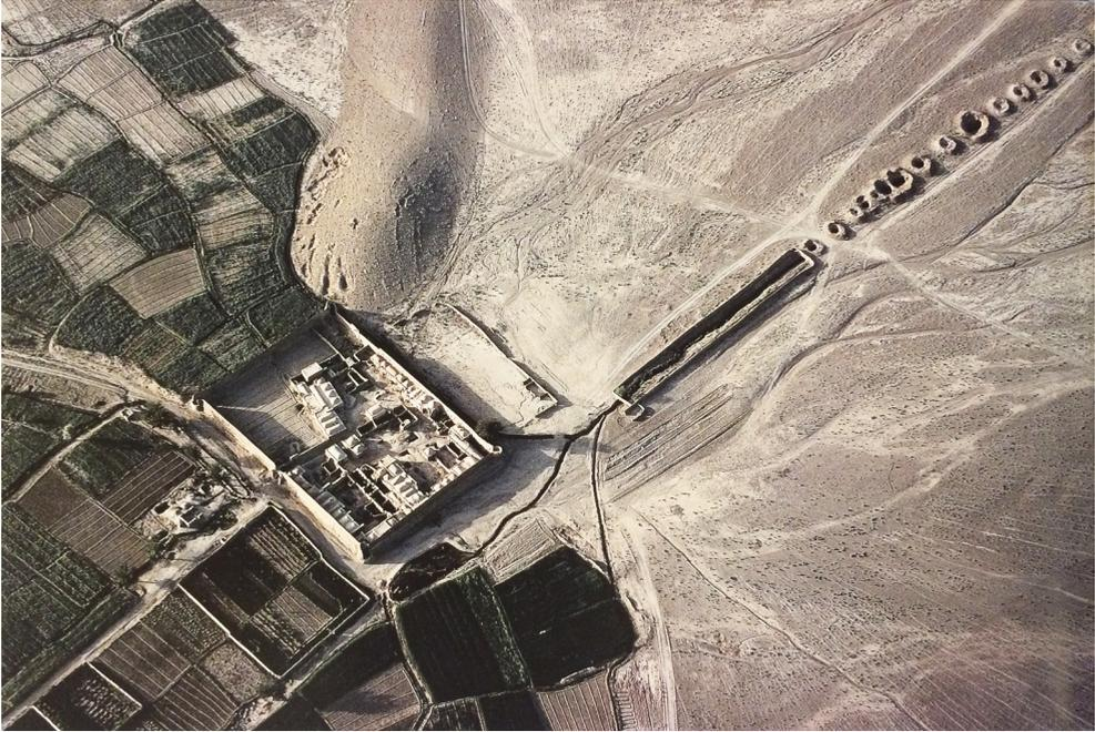
3.10: Golpayegan, Iran. This photo shows the point where ‘a qanat comes to the surface, having carried pristine water deep beneath the bare, uncultivated dasht (whence the word ‘desert’) to its intended destination. Below an initial, walled stretch of the surface stream, three separate irrigation channels then serve to direct the water towards the adjacent fields and settlements.’
