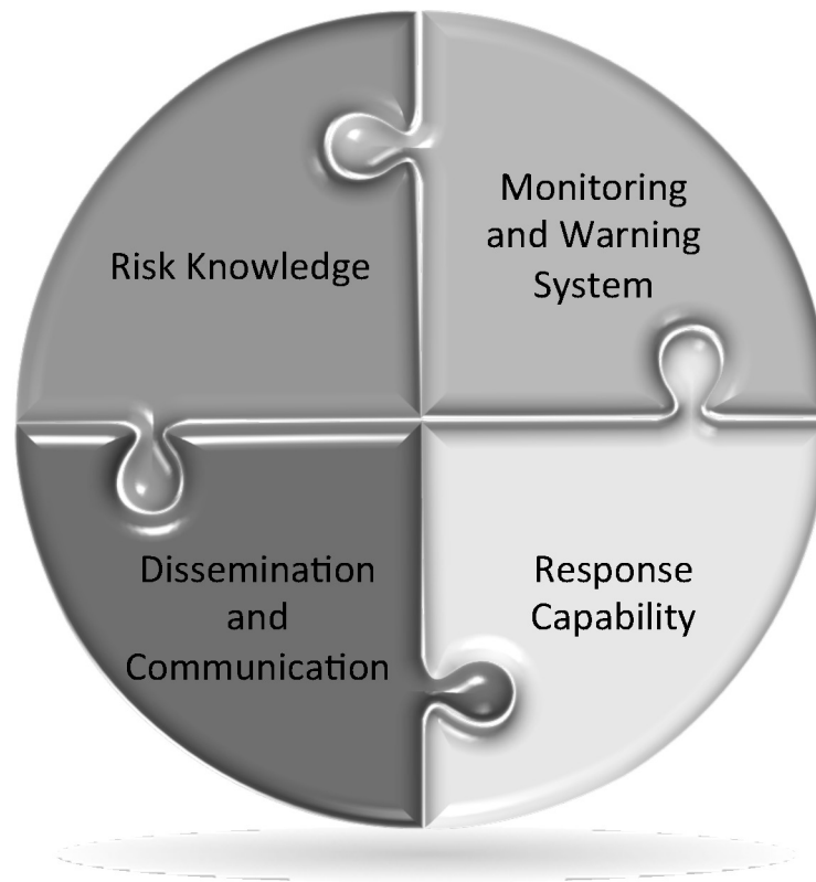
FIGURE 1.1: Flood early warning system components
