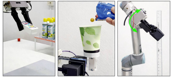
Fig. 7: Overview of the three experimental setups. (1) Object grasping and pivoting [17]. (2) Control stable grasp under increased weight. (3) Rotation experiment with free rotational degree of freedom.
