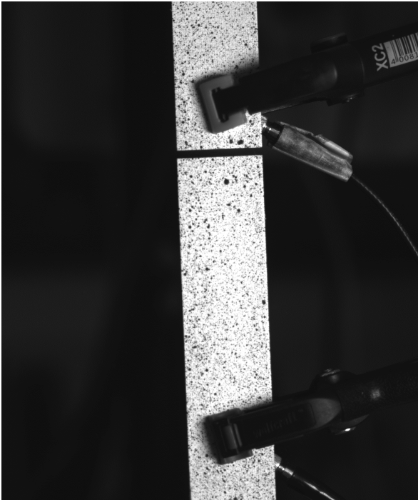
(a) UD specimen after failure
