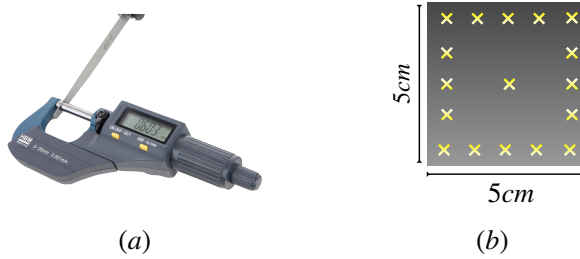
Figure 2.3: ASTM procedure to measure thickness of polymer films. (a) HBM Digital Outdoor Micrometer. (b) Thickness measuring technique. Image of the micrometer retrieved from https://www.hbm-machines.com/nl/
