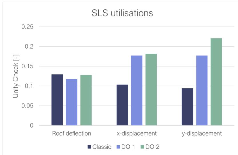
**Figure 6.5:** Geodesic Gridshell with Denser Grid: Displacement utilisation (SLS, 20 m span, C30, 150x125 mm)
