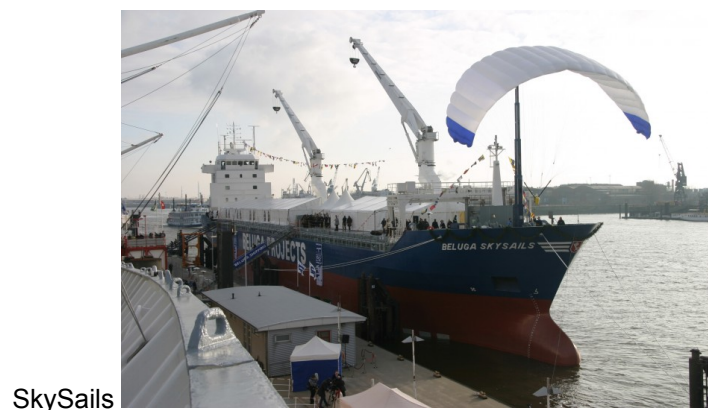
Figure 4.7: A mooring ship retrofitted with a towing kite WPT From MV Beluga SkySails, by Marine Service Noord ( https://marine-service-noord.com/en/projects/mv-beluga-skysails/ )
