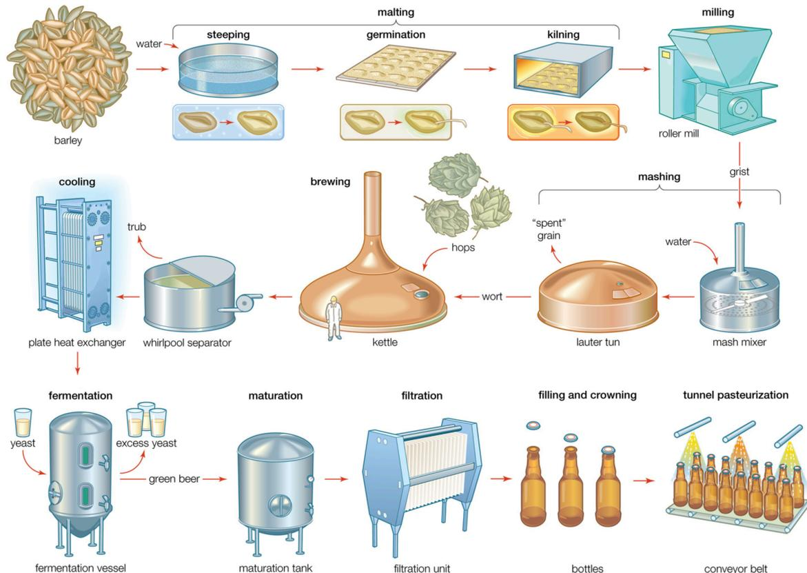
**Figure 2 Schematic representation of the brewing process, from raw material to final product.** Barely is malted, milled, mixed with water and heated to make wort. Hops are added and wort is cooked. Cooled wort is fermented and beer is stored for maturation. Finally, beer is filtered, bottled, and pasteurized. Adapted from Encyclopedia Britannica.
