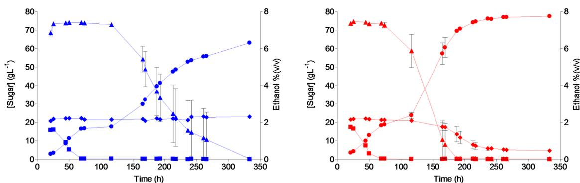
**Fig 5: Extracellular metabolite profiles of *S. eubayanus* strains CBS 12357<sup>T</sup> and IMS0750 in high-gravity wort at 7-L pilot scale.** Fermentations were performed on wort with a gravity of 16.6 °Plato. The average concentrations of glucose (■), maltose (▲), maltotriose (◆) and ethanol (●) are shown for duplicate fermentations of CBS 12357<sup>T</sup> (blue) and IMS0750 (red). The average deviations are indicated (Supplementary data file 7).
