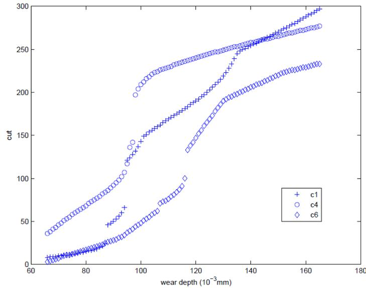
Figure 9: Maximum safe cuts for c1, c4 and c6 [4]
