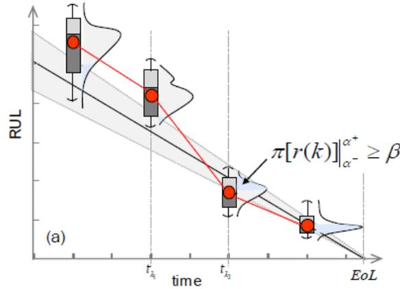
Figure 3:  $\alpha - \lambda$  accuracy cone with the cone shrinking over time [22]
