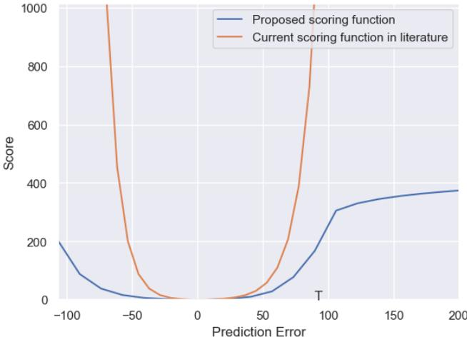
Figure 3. Proposed scoring function with a tolerance of 90 cycles in comparison to the current scoring function
