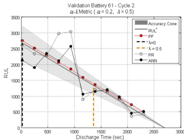
Figure 3:  $\alpha - \lambda$  metric plot for comparison of algorithmic performance [23]
