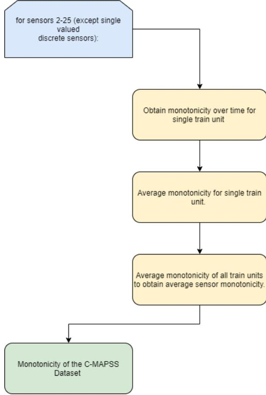
Figure 7. Methodology used for calculating the monotonicity of the C-MAPSS dataset
