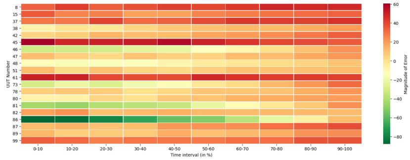
(c) Magnitude of errors throughout the life of the UUTs (generalized linear model)
