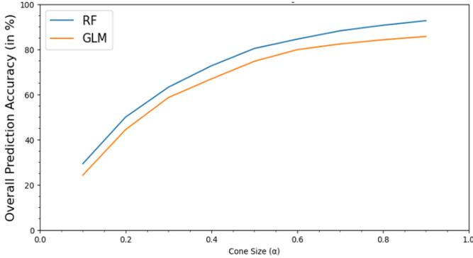
Figure 15. Variation of overall  $\alpha - \lambda$  accuracy with cone size  $\alpha$
