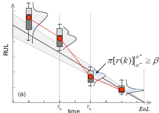
Figure 15:  $\alpha - \lambda$  accuracy with the accuracy cone shrinking with time on RUL vs. time plot [22]
