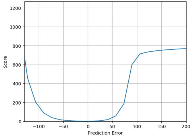
Figure 10. Scoring function as a function of error with  $a_1 = 20$ ,  $a_2 = 14.03$  and  $T = 91$  cycles
