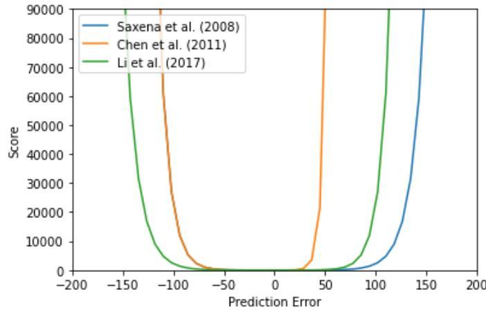
Figure 1: Score as a function of prediction errors for scoring functions highlighted in [20], [4] [13]
