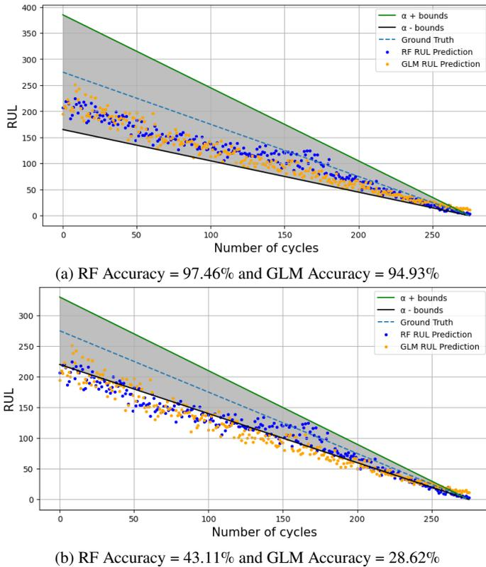
Figure 8. Changes in prediction accuracy with variation of  $\alpha$  for UUT 5
