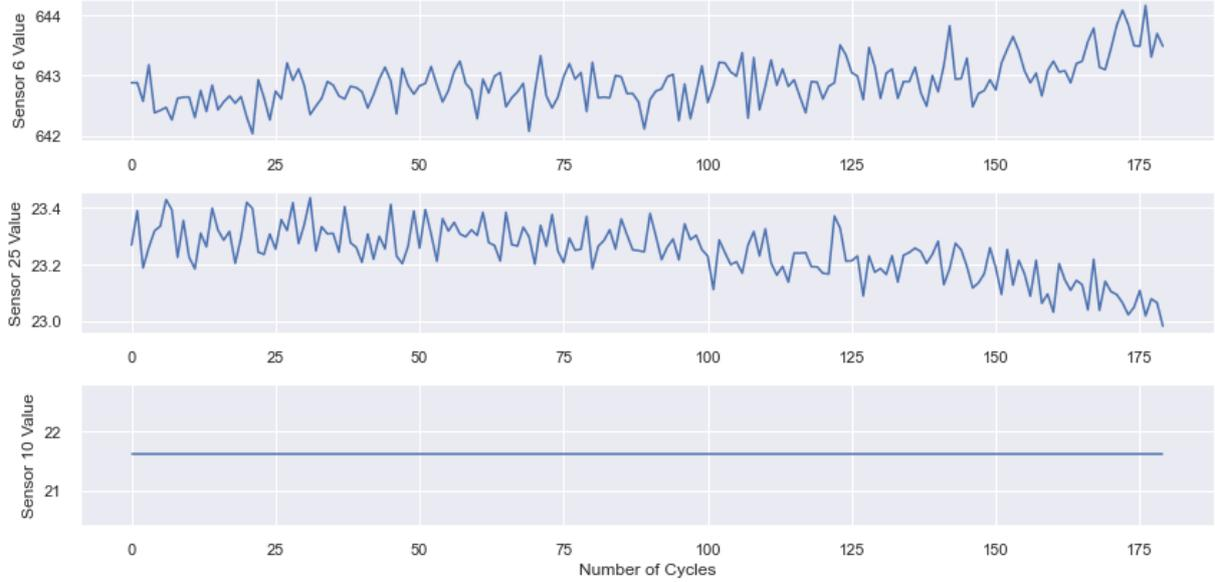
Figure 4. Non-monotonic trends of sensors 6 & 25 with monotonic trend of sensor 10 in C-MAPSS
