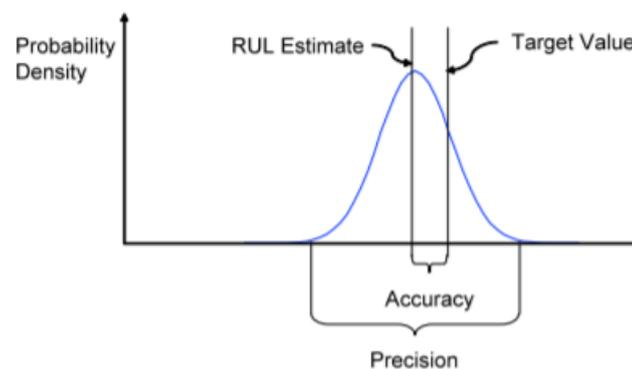
Figure 13: Illustration of accuracy and precision for RUL [29]
