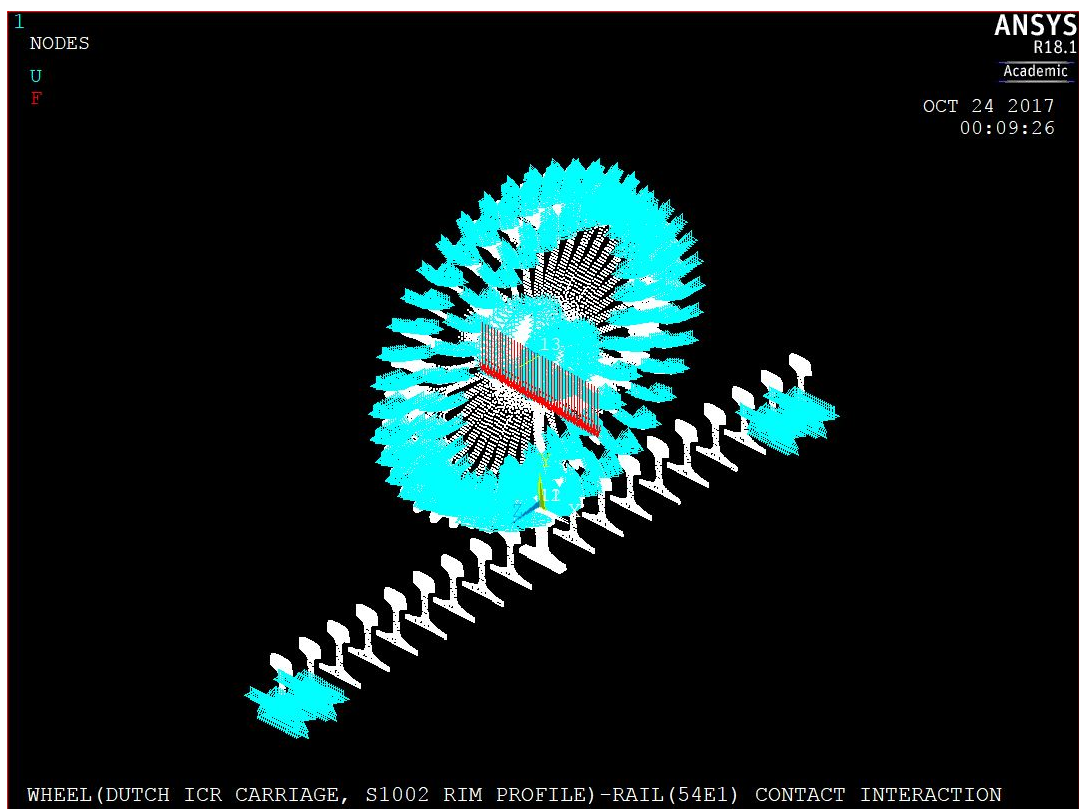
Figure 3.8: Distributed force and boundary conditions
