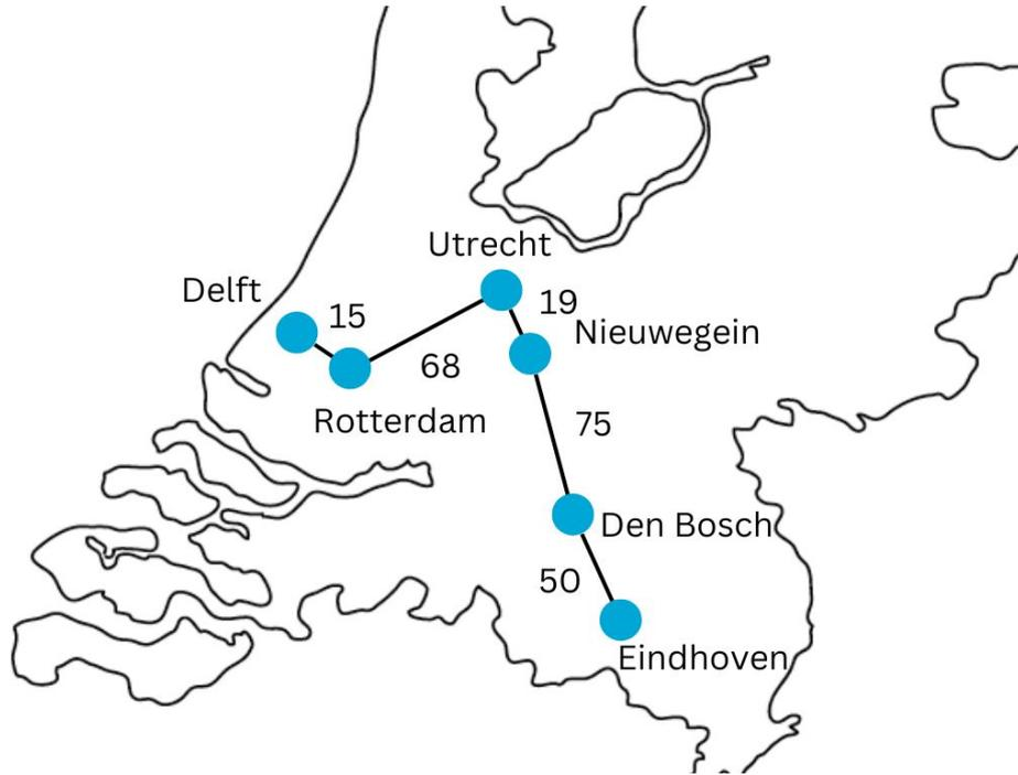
**Figure 5.1:** Schematic depiction of a network based on SURF's fiber infrastructure. The blue circles represent the locations of hubs in the network that possess the facilities to realise quantum hardware. The placement of end nodes, repeater nodes and heralding stations is restricted to these hubs. Distances are in kilometres.
