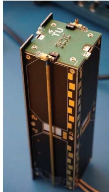
Fig. 1. Assembled 3 unit(3P) Delfi-PQ.
