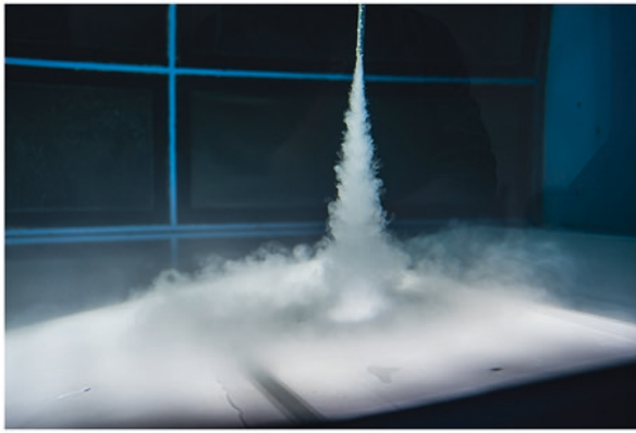
Fig. 7.9 Impression of impinging return flow on inclined floor
