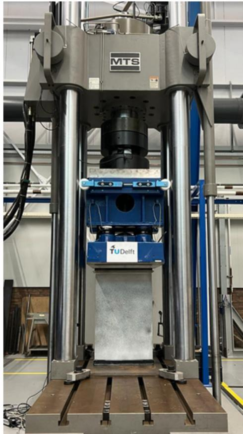
**Figure 6.1:** The mechanical testing setup to use for axial compression testing.
