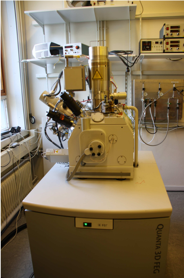
Figure 1.1: The Ga-FIB Quanta™ 3D FEG from FEI; this ‘dual beam’ machine is in the laboratories of the Charged Particle Group at Delft University of Technology.
