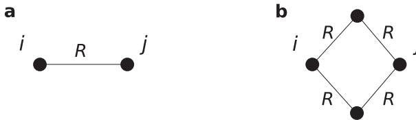
Figure 5.8: Example of two connection patterns with equal effective resistance. Example of two nodes i and j that are (a) connected or (b) not connected and located at opposite sides of a quadrangle. If each link has a resistance R , in both cases the effective resistance \omega_{ij} = R . Thinking of the two graphs as electrical circuits, in graph (a) we simply have one link with resistance R . In graph (b), we have two series connections of length 2 in parallel, each with resistance 2R , that together have effective resistance R .
