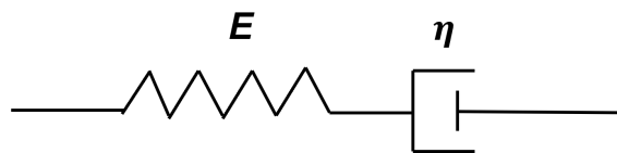
Figure 2.14: Maxwell model—a dashpot with viscosity \eta and a spring with elastic modulus E in series experiencing a stress \tau on both ends. This Figure is self-made, but inspired from[91]
