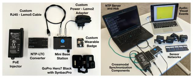
(a) Core components in our setup depicted only with custom cables; (b) Full working setup of our data acquisition system, here the connectors are aligned with the corresponding sockets.
