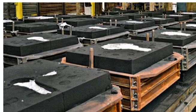
figure 26: Typical use of furan as binder for sand casting moulds (vietnam-castiron.com)
