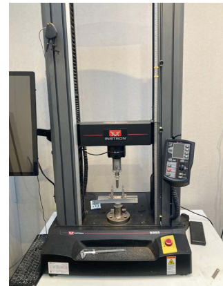
figure 37: UTM with 3-point bending setup
