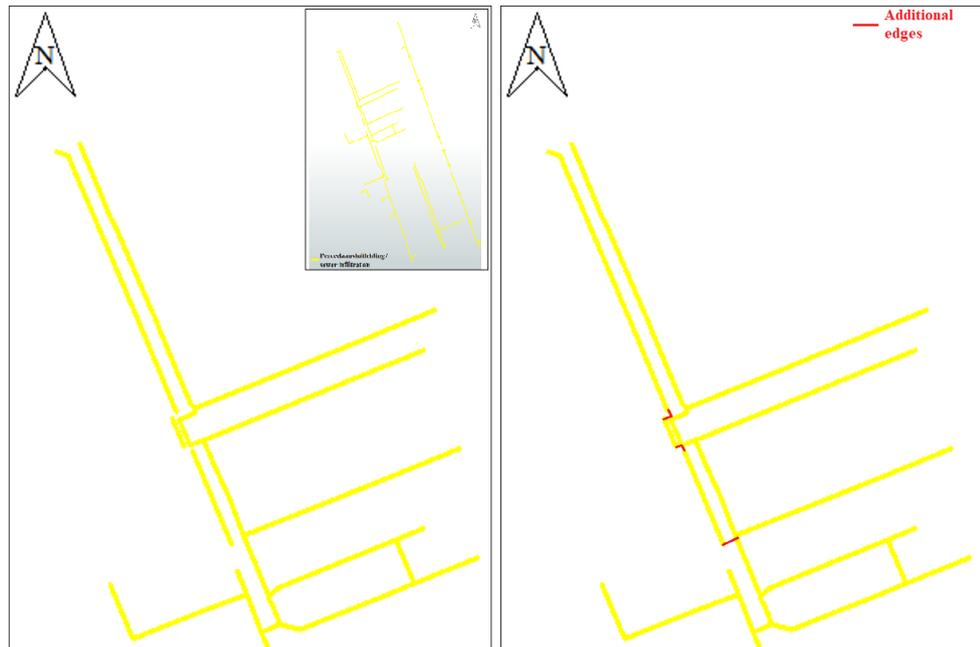
Figure 4.10: Example of manually digitized edges- infiltration network
