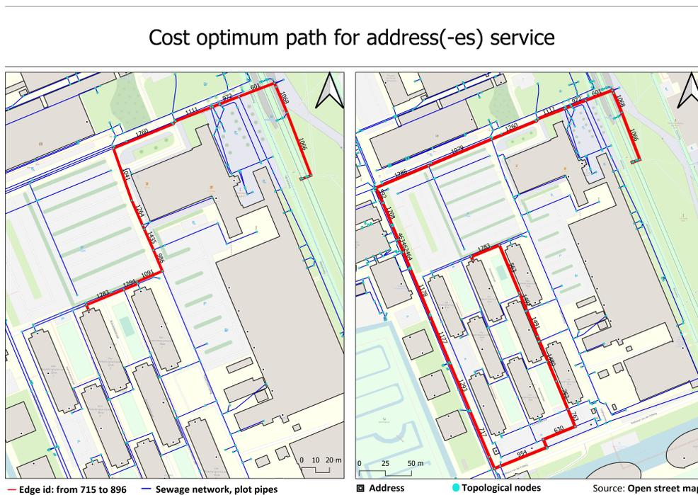
Figure 5.13: Cost-optimum path detection- addresses dataset
