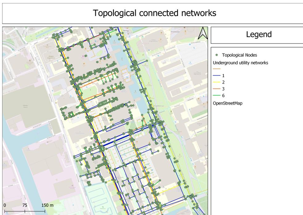
Figure 5.3: Topologically reconstructed network
