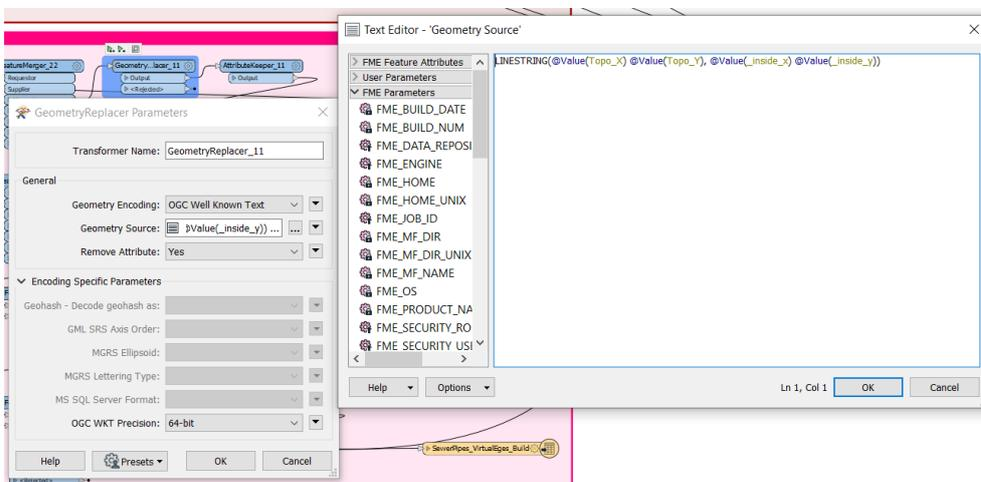
Figure 7.2: FME workspace example- virtual edges creation
