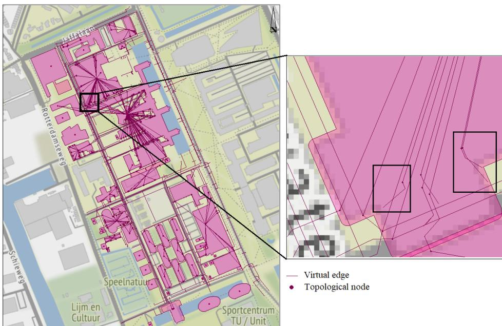
Figure 4.18: Example of topological node simplification
