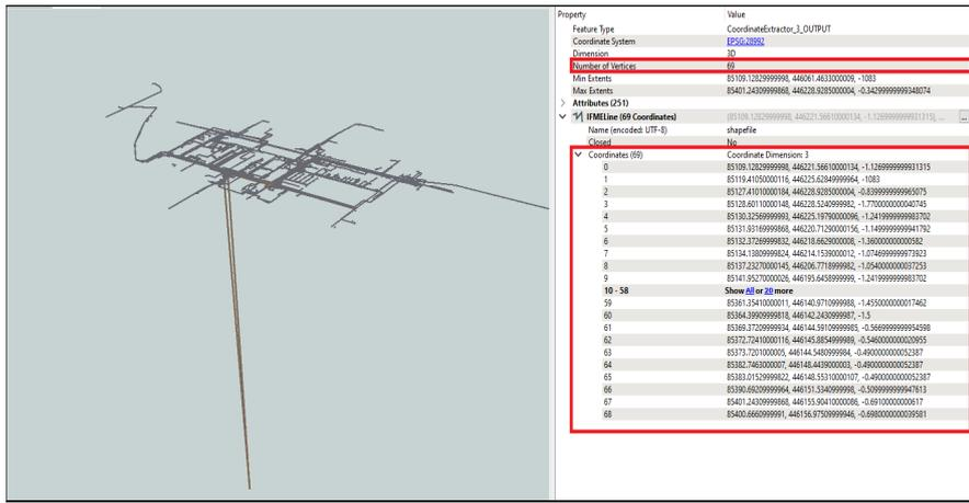
Figure 3.8: Incorrect topology derived from incorrect, input, attribute
