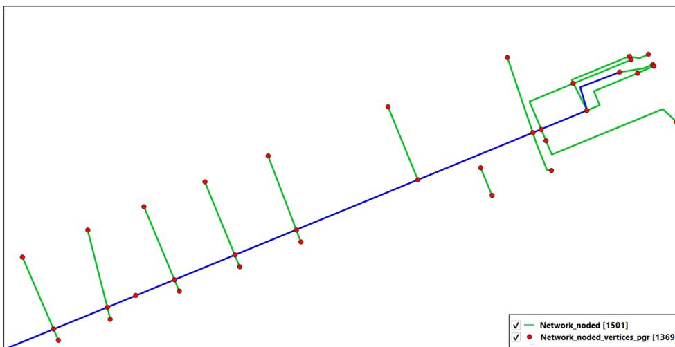
Figure 5.6: Topological edges (sewage-plot pipes networks) **after** pgRouting algorithms implementation
