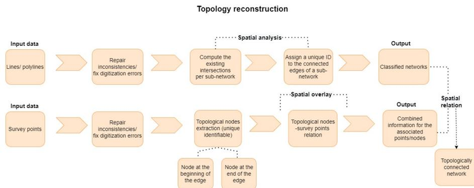
Figure 3.17: Topology reconstruction flowchart
