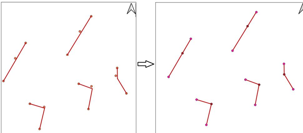
Figure 3.16: Example of fixing digitization errors- network elements
