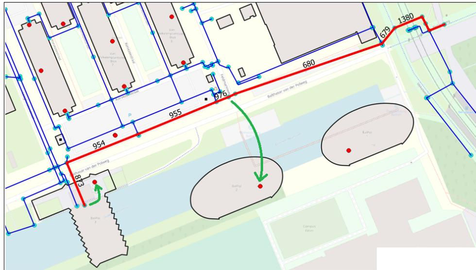
Figure 5.11: Addresses points associated with the nearest topological nodes
