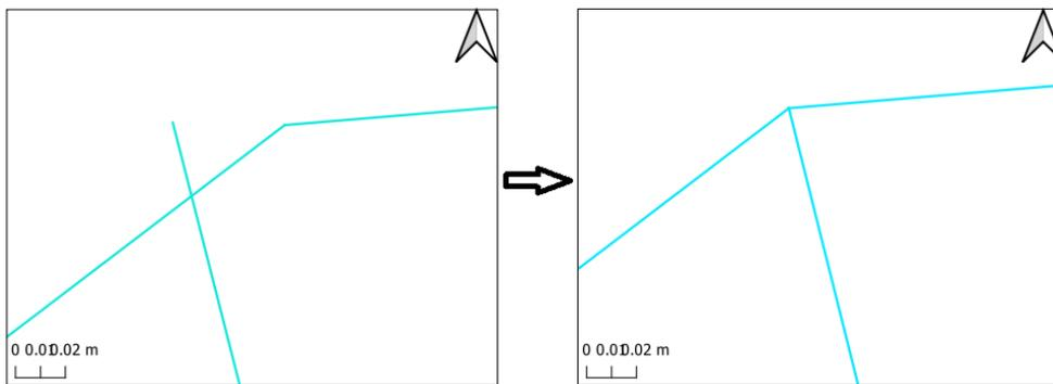
Figure 3.15: Example of fixing digitization errors- network
