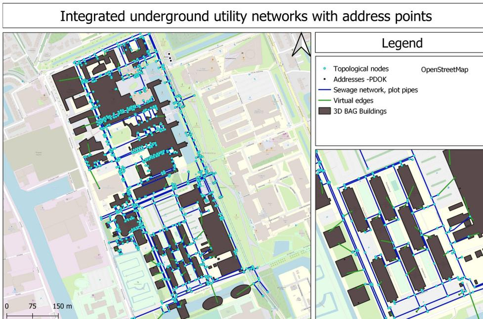
Figure 4.24: Example of virtual edges between address points and topological nodes
