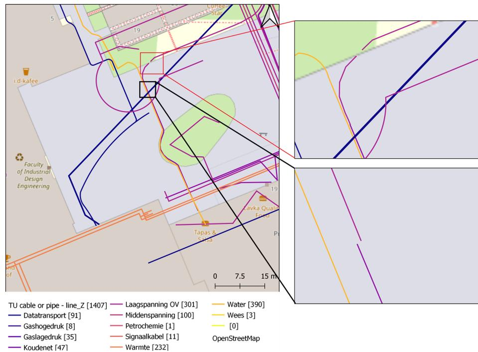
Figure 3.13: Example of topological inconsistency- dis-junction
