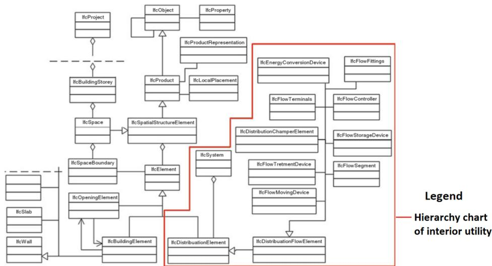
Figure 2.3: IFC inside building utility network schema
