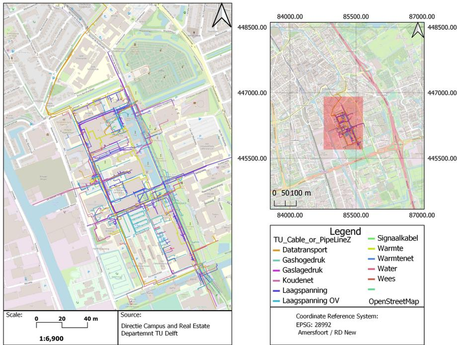
Figure 3.3: TU cable/ pipes network (e.g gas, electricity)
