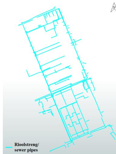
Figure 4.4: Rioolstreng/ sewer network
