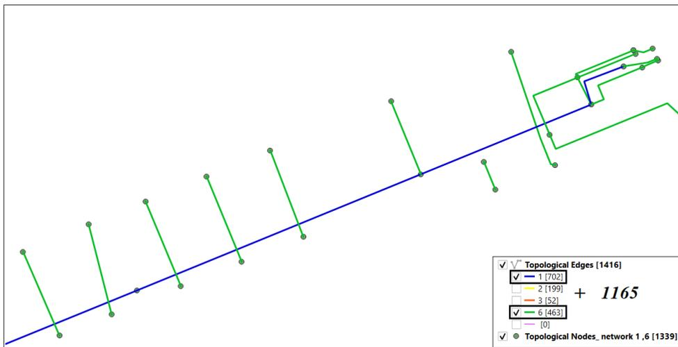
Figure 5.5: Topological edges (sewage-plot pipes networks) **before** pgRouting algorithms implementation
