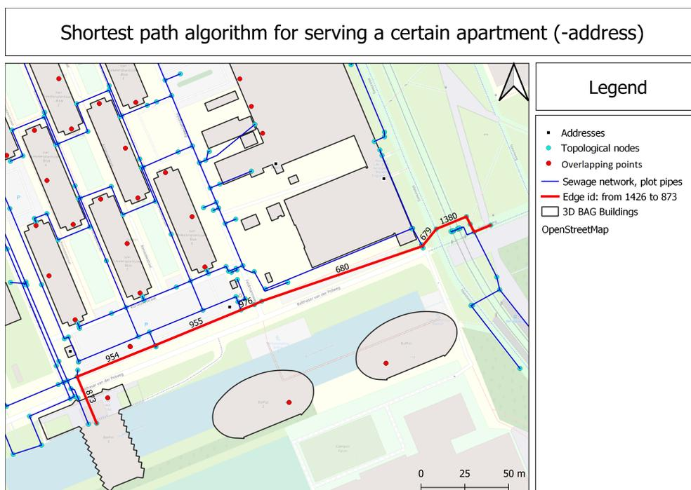
Figure 5.10: Example of optimum path and the affected addresses in case of disaster
