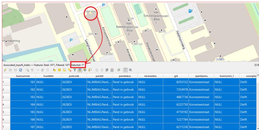
Figure 4.23: Example of overlapped points with different house numbers
