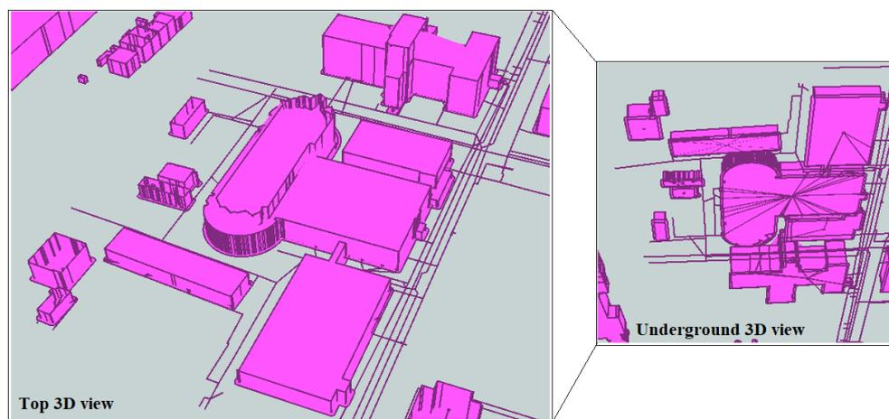
Figure 4.19: 3D representation of buildings and underground utility network
