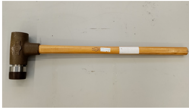
Figure 3.7: The impact hammer used
