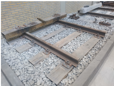
Figure 3.8: Track structure used in experiment
