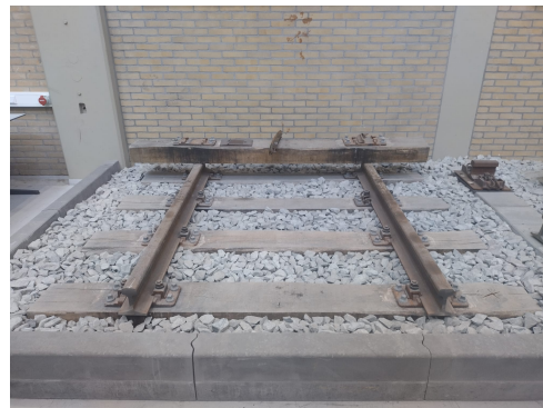
Figure 3.9: Track structure used in experiment
