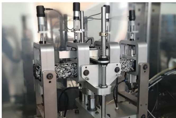
Fig. 7. The beam fatigue test setup.
