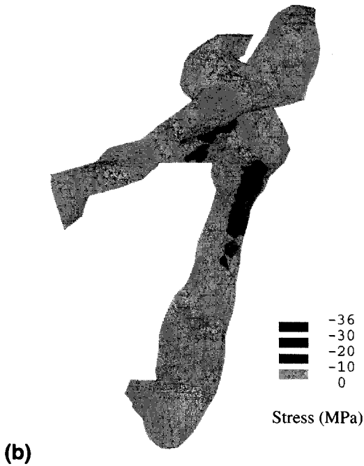
Figure 6. Principal normal (compressive) stress distribution (MPa) during 90-degree humeral abduction (dorsal view); (a) shell elements; (b) solid elements.
