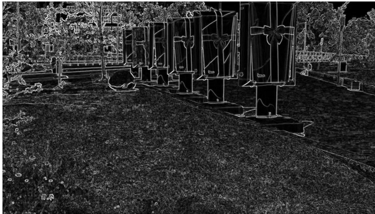
Figure 3.5: Built-in OpenCV Sobel filters applied to boxes.png and plotted for magnitude
