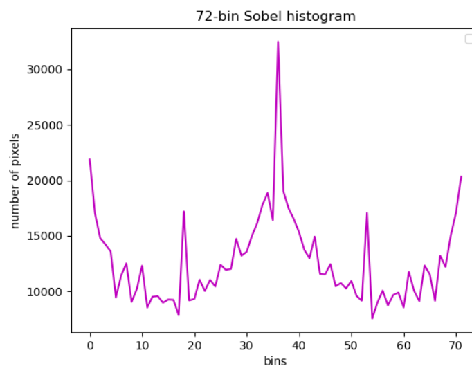
Figure 3.6: Corresponding 72-bin (180 degrees) Sobel histogram
