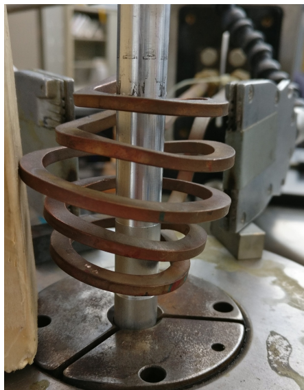
Figure 4.7: The Ultra High Frequency heating setup
