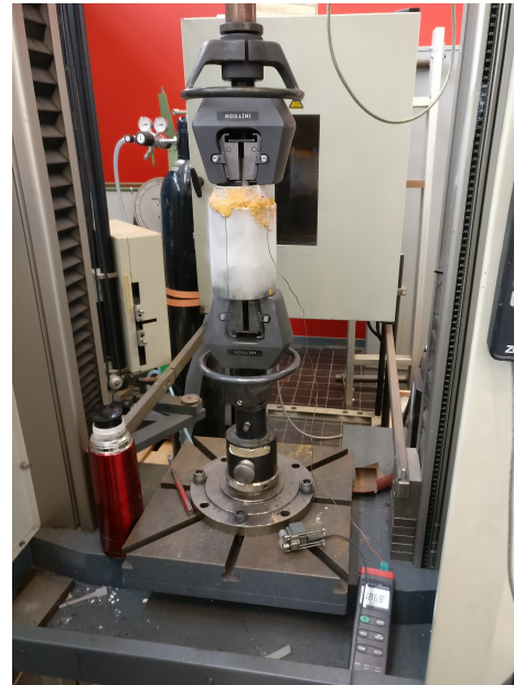
(b) The AALT method, the specimen is cooling in the nitrogen tank
