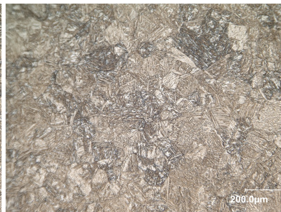
Figure C.17: CGHAZ microstructure from the edge of the bar (250x)
