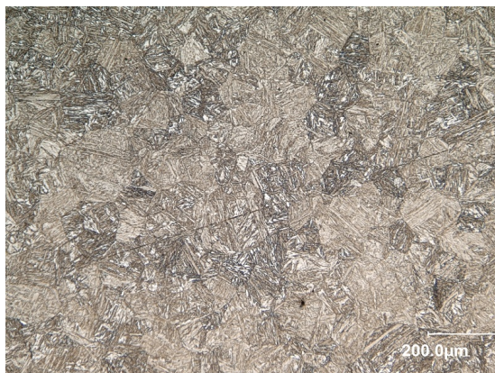
Figure C.16: CGHAZ microstructure from the center of the bar (250x)
