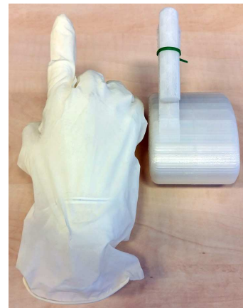
Fig. 5. Attachments used in conditions PHI (left) and nPHI (right). Note that the attachment of the nPHI-setup does not include a hand and that a tie-wrap is strapped around the finger-like boom; both to accentuate the non-human physique.
