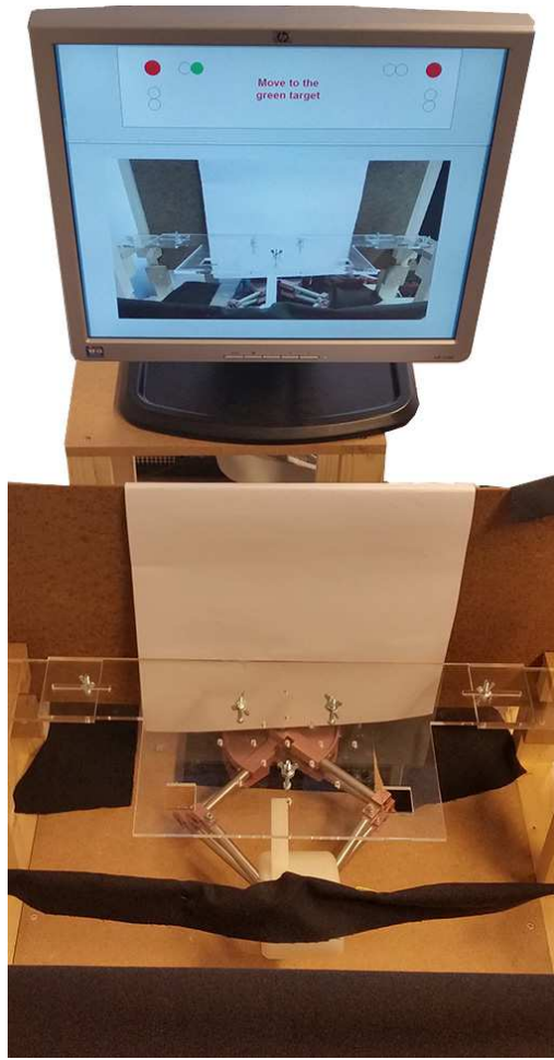
Fig. 3. Front view of the master-side setup. At the bottom the attachment and the small cloth curtain are visible, with right above the attachment the transparent obstacle plate, holding the three obstacles. The monitor with the visuals presented to the participant during the experiment is visible at the top.
