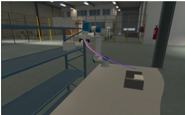
Figure 4. Virtual Reality trajectory projection example
