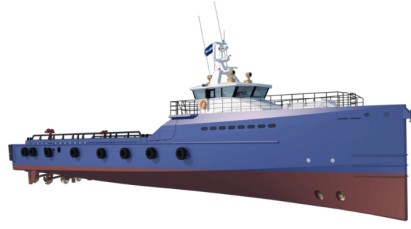
Figure 7: Render of the fast crew supplier 5009 by Damen ([2])
