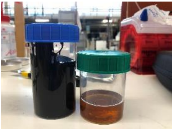
Figure 21: Epoxy resin used for insulation of connection, with polyurethane resin at the left, and hardener at the right, purchased from Electrolube
