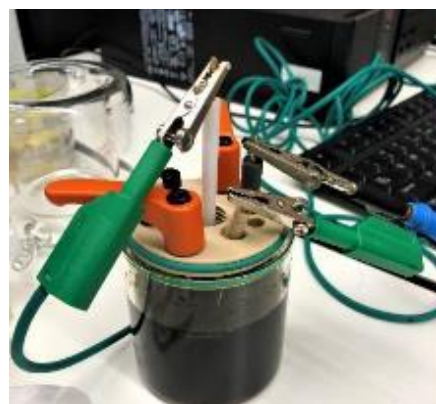
Figure 13: Electrodeposition cell setup, with all three electrodes and crocodile clips to connect them to the potentiostat
