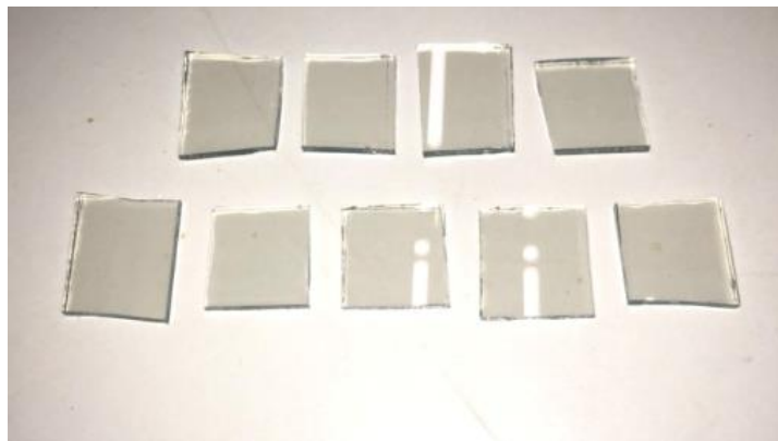
Figure 50: Multiple FTO substrates cut into an area of 4 cm by 4 cm
