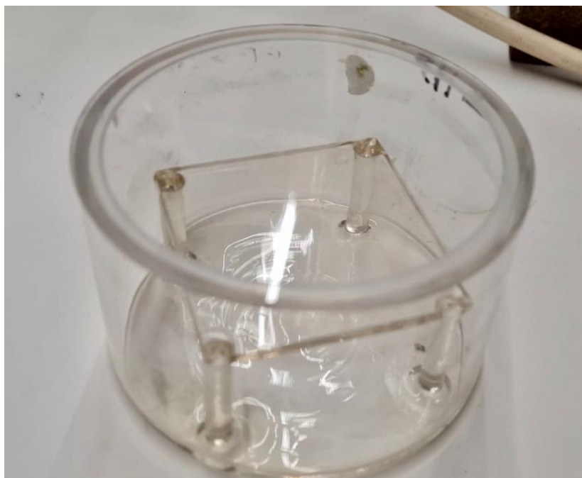
Figure 54: Reactor cell used for degradation experiments (175 mL capacity)
