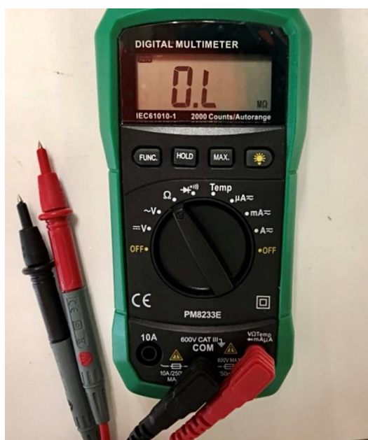
Figure 51: Digital multimeter used to indicate the conducting FTO side of the glass substrates
