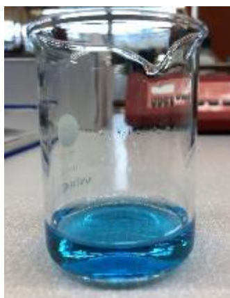
Figure 10: Precursor solution for dip-coating
