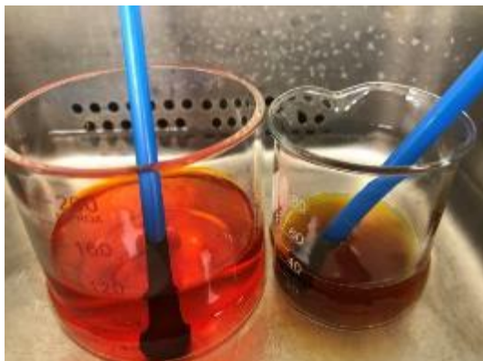
Figure 12: Precursor solutions for electrodeposition. The one on the left is KI and \text{Bi}(\text{NO}_3)_3 \cdot 5\text{H}_2\text{O} in demineralized water, and the one on the right is para-benzoquinone in ethanol
