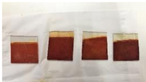
Figure 14: BiOI electrodes produced at -0.2 V at different times of electrodeposition
