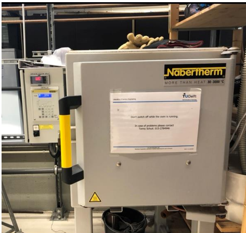
Figure 53: Furnace (Nabertherm) used for annealing the \text{BiVO}_4 electrodes
