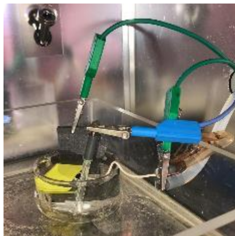
Figure 24: Reactor cell setup for PEC, with all three electrodes and the electrolyte with the OMP
