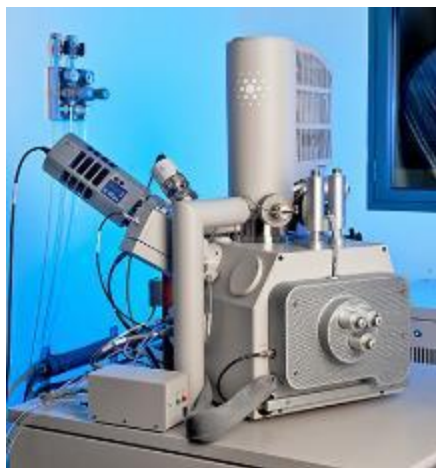
Figure 17: Illustration of the microscope for SEM (FEI Model Quanta 650), used to study the surface morphology of the BiVO 4 electrodes
