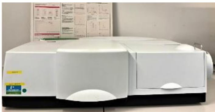
Figure 18: LAMBDA 1050+ UV/Vis/NIR spectrophotometer used to study the absorption behavior of the \text{BiVO}_4 electrodes
