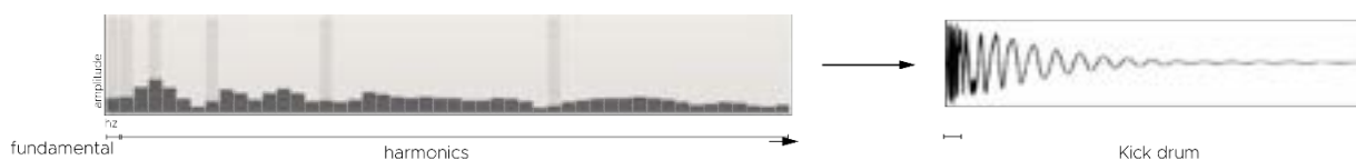
Figure 1: Additive synthesis. Every bar is a sine wave at different frequencies. (Own Image)
