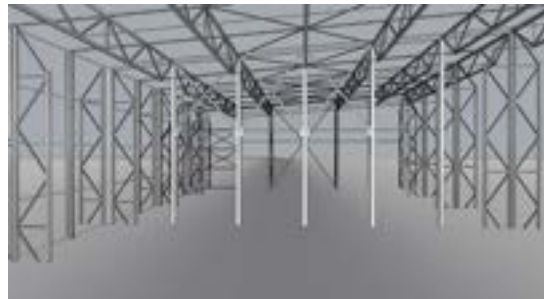
To make the hall more of a continuous space, where the stability crosses are not in the way, I want to change them in the middle part to this. The image above shows the new version.
