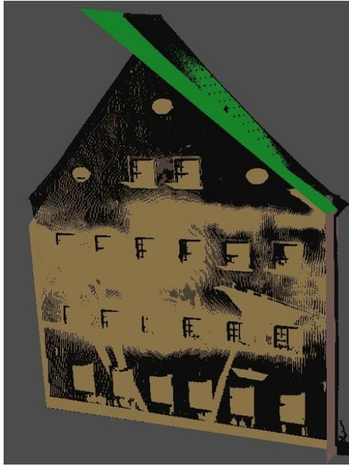
Figure 18: Planes segmented by refined RANSAC algorithm
