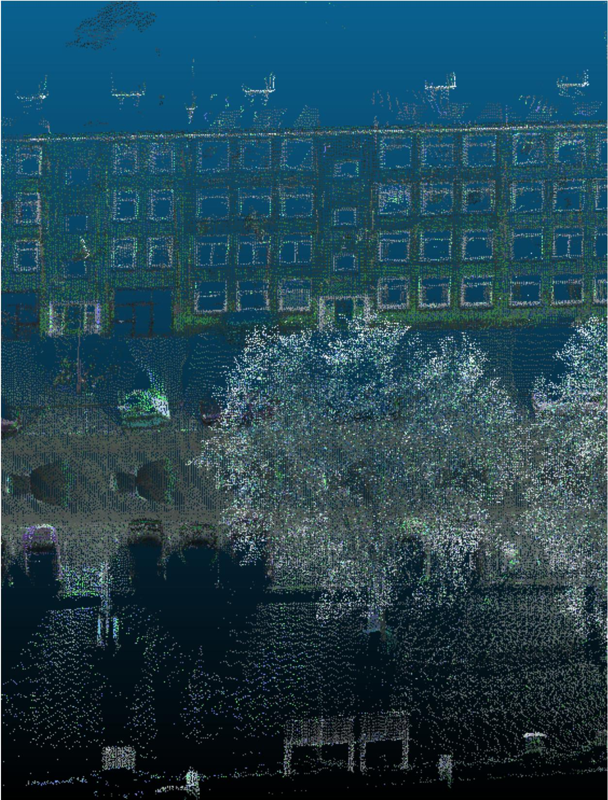
Figure 47: Point cloud subset before ground filtering
