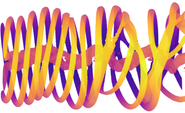
(a) Top-view Q-criterion ( Q = 3.5 \times 10^{-3} \text{ s}^{-2} ) of case 4 ( 5^\circ , 0.05Hz, TSR 7).
