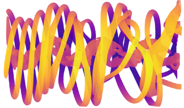
(b) Top-view Q-criterion ( Q = 3.5 \times 10^{-3} \text{ s}^{-2} ) of case 5 ( 10^\circ , 0.05Hz, TSR 7).
