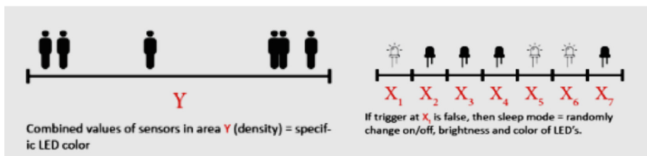
Fig. 4. Design scheme for a dynamically responsive lighting system based on automated inputs was linked real-time to user activities such as seating, walking, running.
