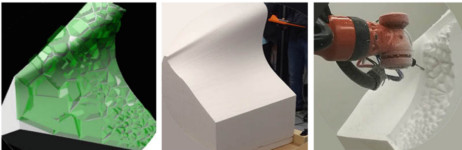
Fig. 3. D2RP process linking parametric 3D model (left) with robotic hot wire cutting (middle) and milling (right).
