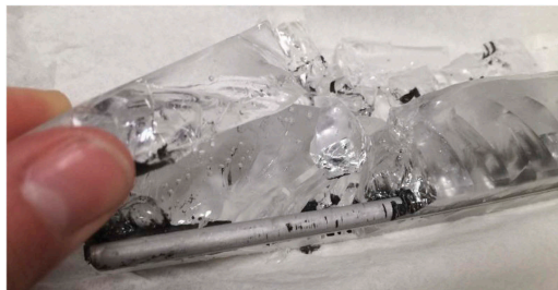
Figure 8. Upon glass failure, the separation of the two materials can be mechanically achieved.
