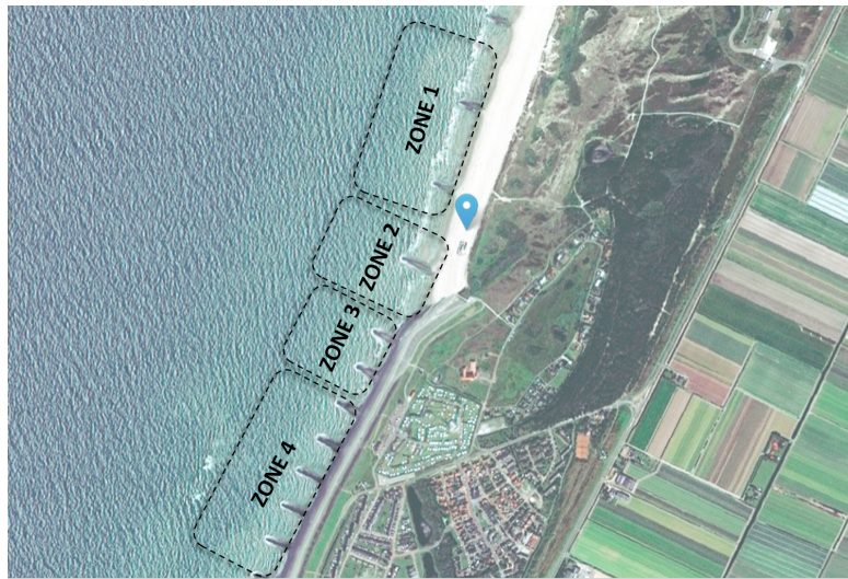
Figure 6.7: Visualisation of the general morphological behaviour of hard-soft transitions, here applied to the old Hondsbossche- and Pettemer Zeewering (HPZ).
