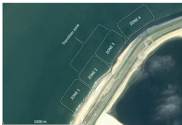
Figure 6.6: Visualisation of the morphological behaviour at the hard-soft transition of MV2
