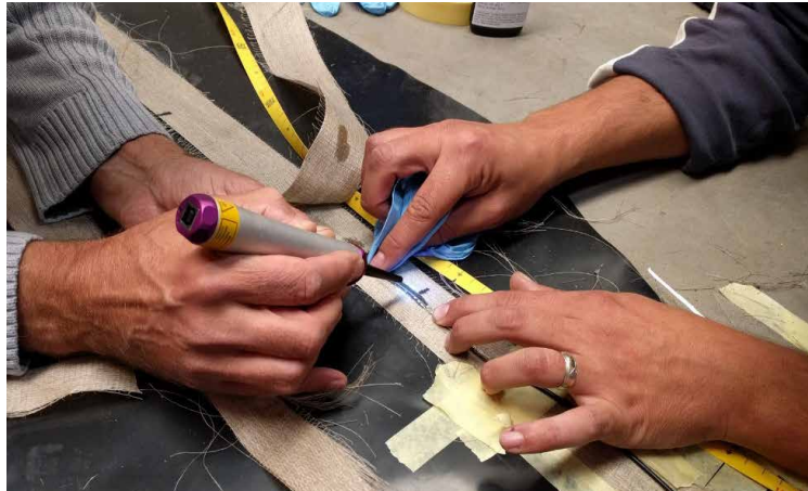
FIGURE 5.11 Preparation of optical (glass) Fibre Brag Grating sensors. R. Blok, J. Smits et al., Eindhoven University of Technology & Delft University of Technology, (2017).
