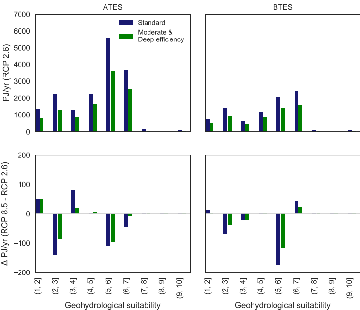
Figure 8.6: Worldwide distribution of estimated energy use in large urban areas in suitable climate zones and relevant building sectors, as a function of geohydrological suitability and building efficiency scenarios, for ATES (left panels) and BTES (right panels). Top panels: RCP 2.6; bottom panels: change in energy use under RCP 8.5 relative to RCP 2.6.
