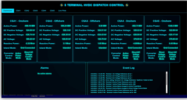
Fig. 5: Web-based dashboard showing terminal-specific data, live plots, and control elements.
