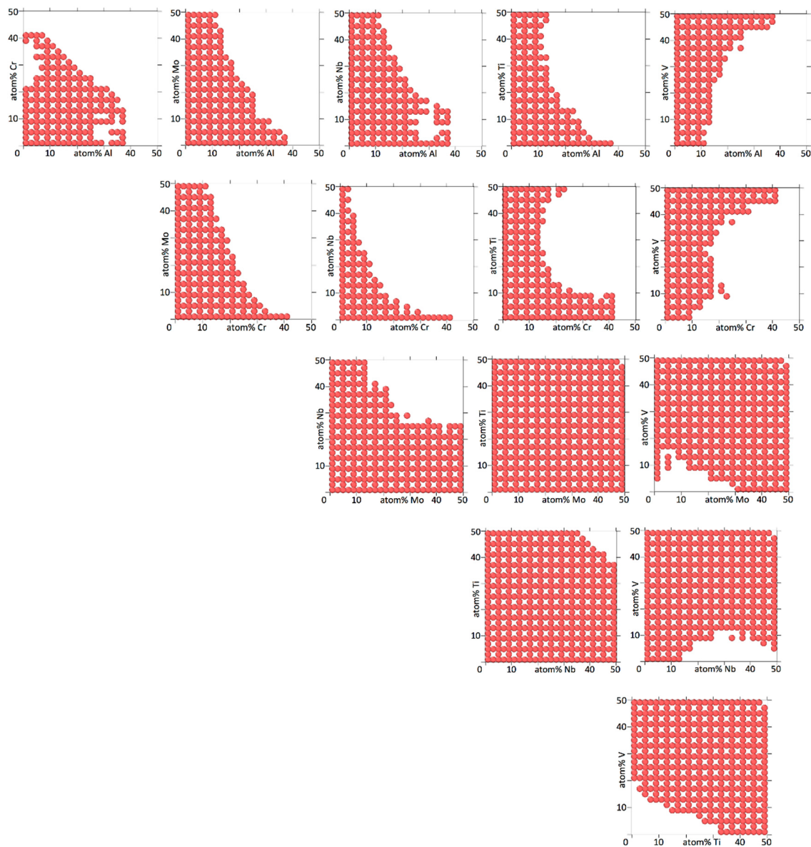
Figure 7. Two-dimensional projections for \text{Al}_a\text{Cr}_b\text{Mo}_c\text{Nb}_d\text{Ti}_e\text{V}_{1-a-b-c-d-e} , showing at which concentrations for two elements the alloy forms a bcc HEA at 800 K. Four concentration dimensions are flattened out to arrive at the two-dimensional projection. The concentrations of the four elements not shown are as explained in the caption of Figure 2. The concentration increments are 4%.
