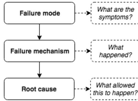
**Figure 4.5:** *Hierarchy in root cause failure analysis*
