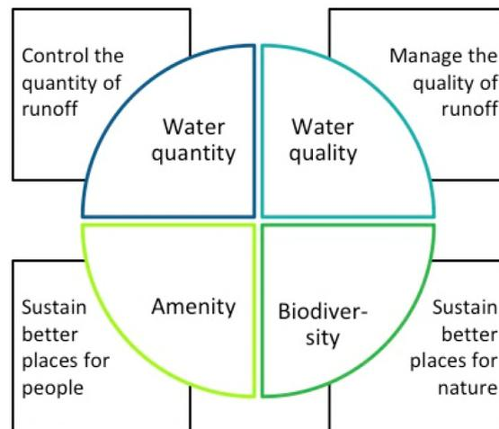
**Figure 2.3:** *Multifunctionality of SUDS described by the coexistence of four pillars (CIRIA, 2015)*
