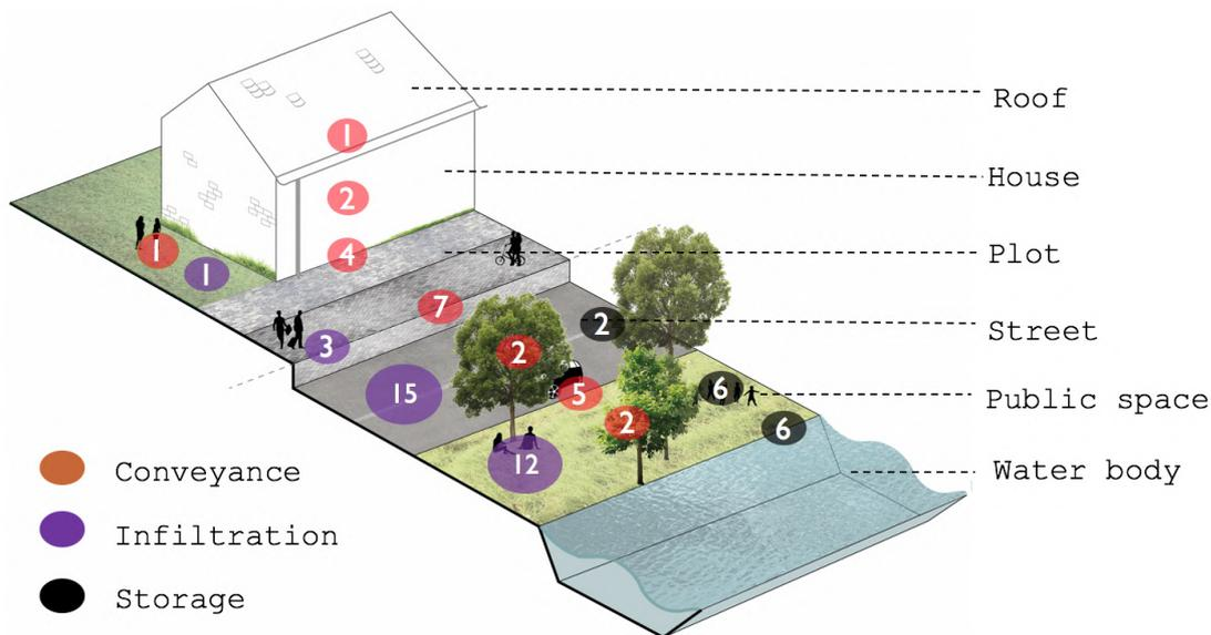
**Figure 7.3:** *The locations of where technical failures occur, specified per SUDS function (conveyance, infiltration, storage). Numbers indicate the number of cases from the data set that fail on that particular location.*
