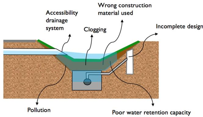
**Figure 7.2:** *Technical failures occurring in a bioswale*
