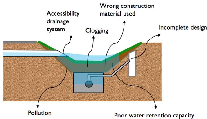
Figure 5.9: Technical failures occurring on the open space
