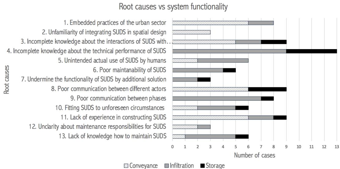
**Figure 5.22:** A combination of the root causes and the SUDS functionality
