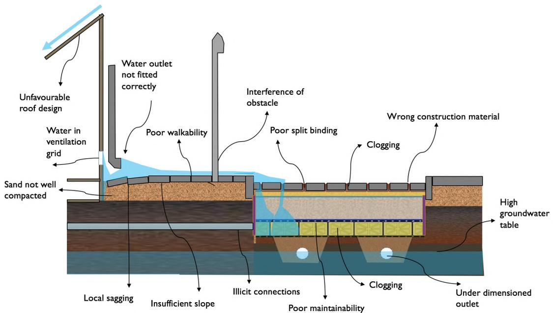
**Figure 7.1:** *Technical failures occurring on the street*
