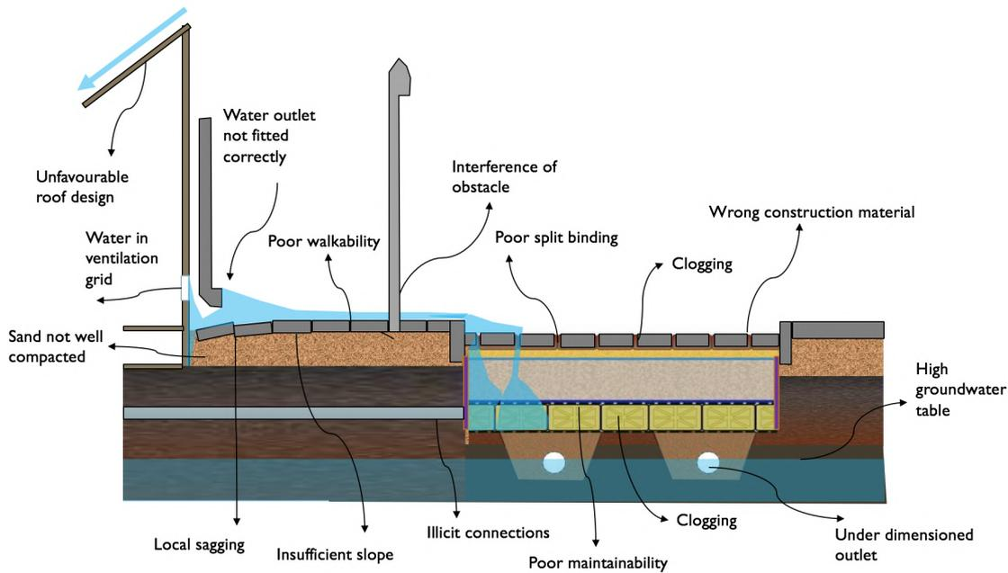
Figure 5.8: Technical failures occurring on the street
