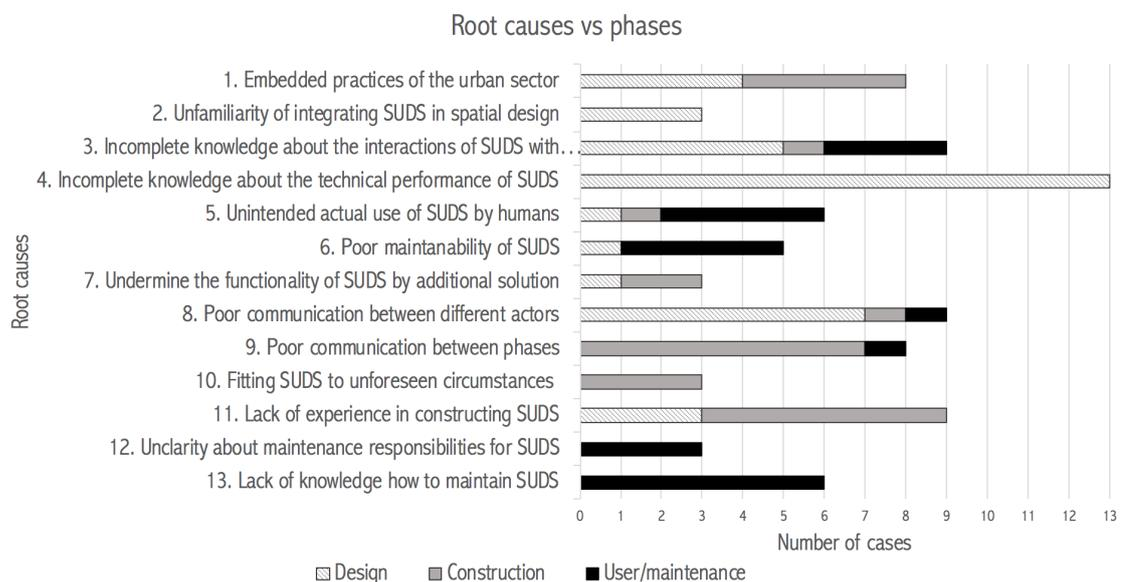
**Figure 5.24:** *The combination of root causes and the project phases*
