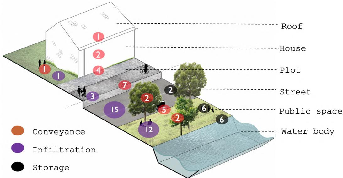
**Figure 5.3:** *The locations & number of the failures specified per SUDS function (e.g. conveyance, infiltration, storage)*
