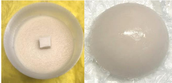
Figure 1: Left: breast mold including healthy phantom tissue up to 20 mm with the cubic tumour phantom on top, Right: The breast shaped phantom with a total volume of 500 mL.
