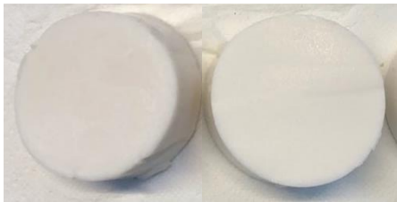
Figure 4: Visual properties of the healthy- (left) and barium sulphate tumour phantom (right), barium sulphate (BS).
