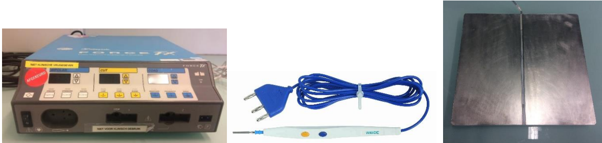
Figure 40: Left: Electrosurgical generator, Middle: electrosurgical knife, Right: Dispersive pad 7 .
