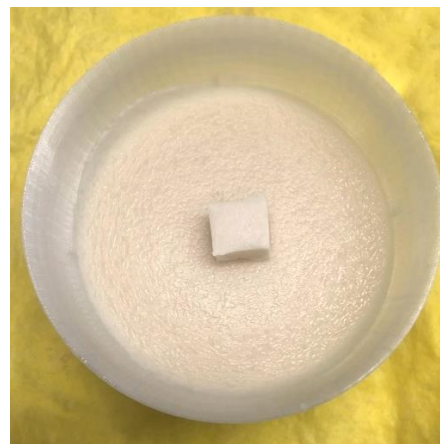
Figure 52: Left: breast mold with a total volume of 500 mL, right: breast mold including healthy phantom tissue up to 20 mm with the cubic tumour phantom on top.
