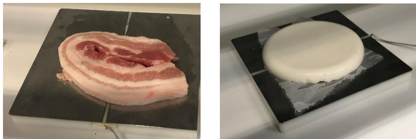
Figure 41: Left: Pork belly on dispersive pad, Right: phantom tissue on dispersive pad.
