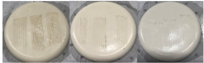
Figure 6: From left to right: the healthy-, tumour- and barium sulphate tumour phantom. Per phantom type, tissue effects from left to right: coagulation, blend cut and pure cut.
