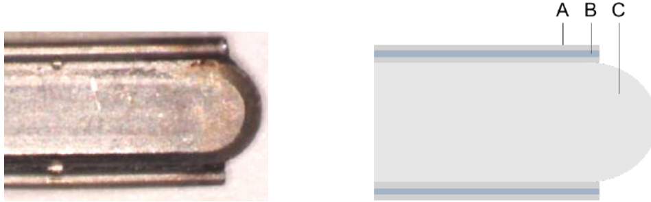
Figure 6: The tip of the cutting blade with two fibres attached to it. Left, a microscopic picture of the prototype 7 . Right, a schematic image of the cutting blade (C), fiber (B) and the metal sleeve (A) 12 .
