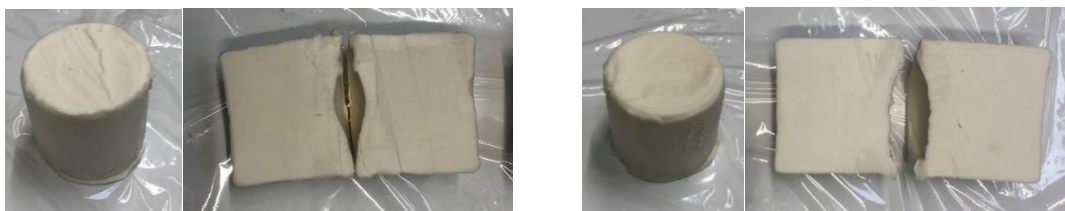
Figure 20: Agar/water/lipid-based phantoms in combination with EL 11 or EL 33: 1 left, 2 right.
