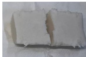
Figure 19: Agar/water/lipid-based phantom with a temperature decrease to 35 °C: 1 left, 2 right.
