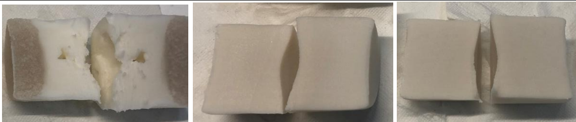
Figure 18: Phantoms with different F/W-ratios and produced with tap water: 4 left, 5 middle, 6 right.
