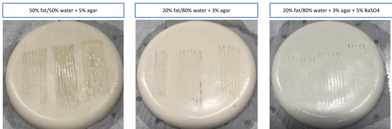
Figure 51: The most potential agar phantoms with and without BaSO 4 . From left to right, tissue effects as a result of coagulation, blend cut and pure cut.
