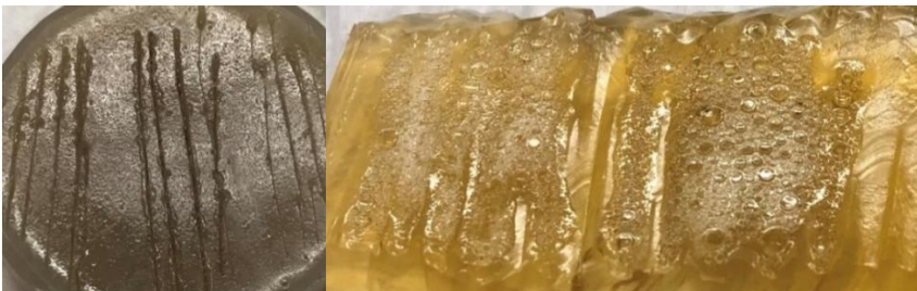
Figure 44: Left pure agar phantom with 5% of agar by weight of water. Right pure gelatin phantom with 20% gelatin by weight of water. From left to right tissue effects as a result of coagulation, blend cut and pure cut.
