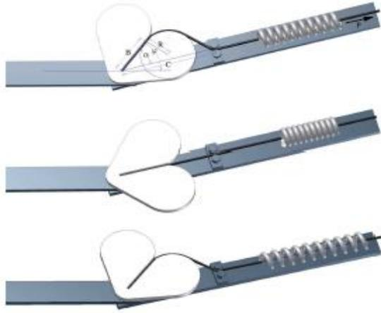
Fig. 4. Working principle of the novel MACCEPA 2.0. Top: Out of equilibrium position (generating torque) Middle: At equilibrium position (not generating torque) Bottom: Changed pretension.
