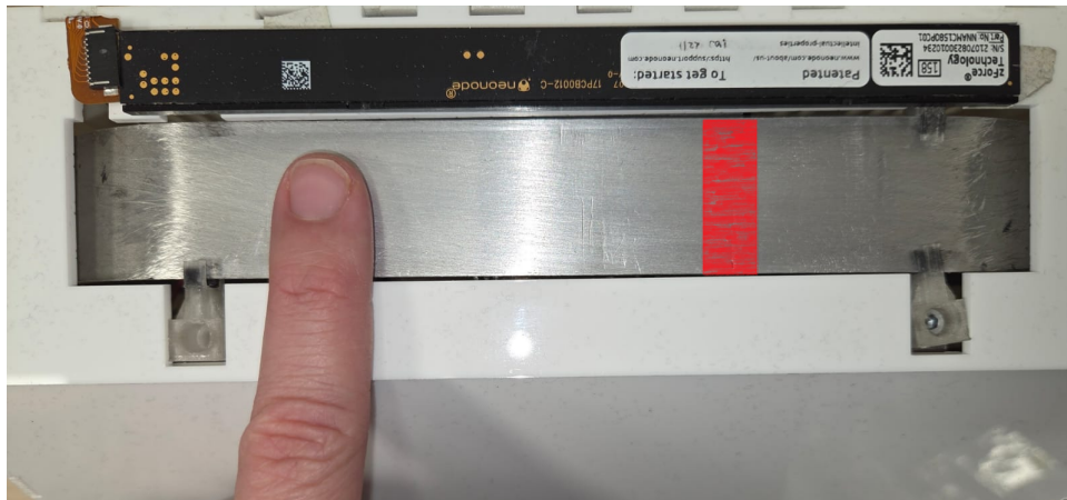
Figure 3.2: The Ultraloop contact surface for the participants to follow the moving virtual target, indicated by the red overlaid rectangle. Also, a position sensor is mounted on top to measure the finger position of the participant.
