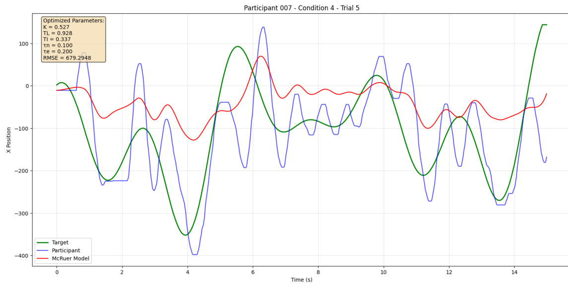
Figure 4.12: Resulting paths generated by the moving target(green), the participant(blue) and the McRuer crossover model(red). Top-right legend displays the optimized parameters for the fitted McRuer model. These results come from participant 007 during condition 4 (No Vision + Active Force Feedback) and movement trial 5.
