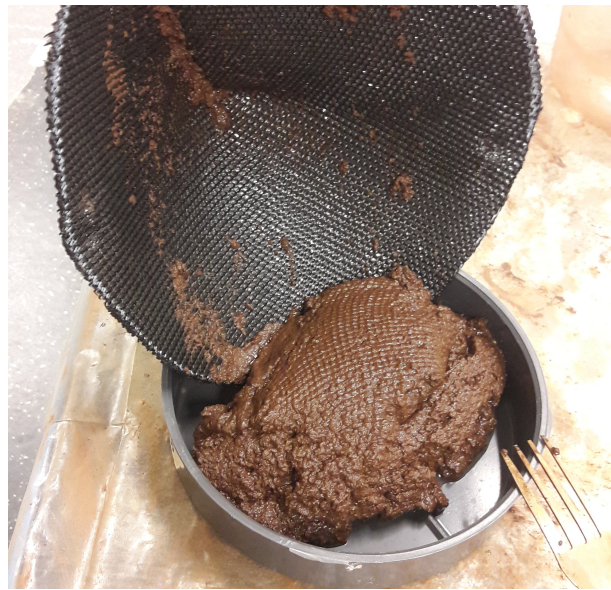
Figure 7.4: Pouring of dewatered slurry in mould.
