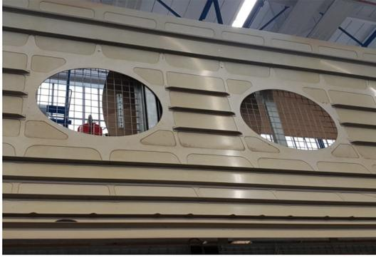
Figure 1.1: Fuselage cutouts for windows
