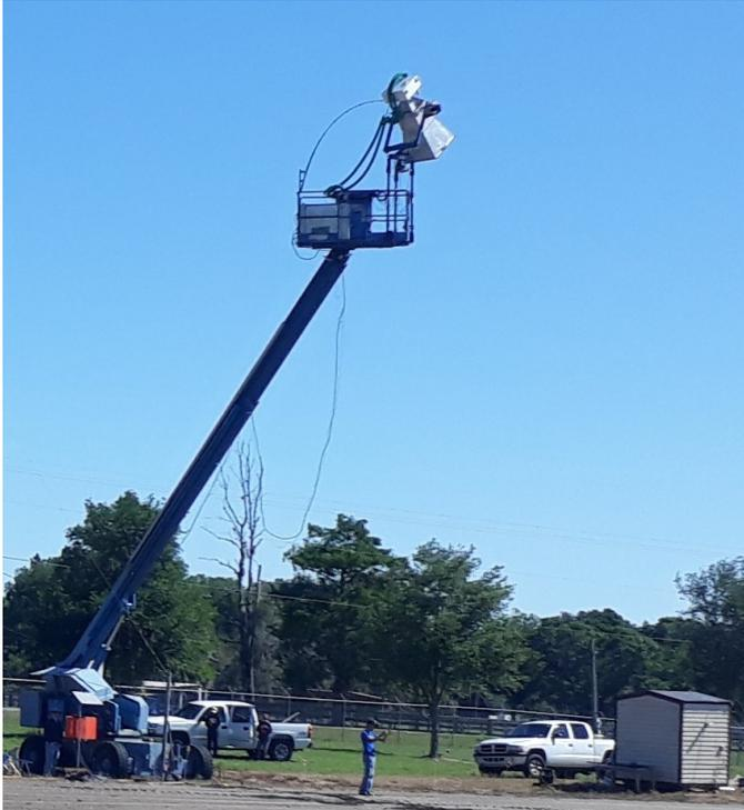
Figure 3.3: UF-LARS in corn field mounted on the 25 m Genie platform
