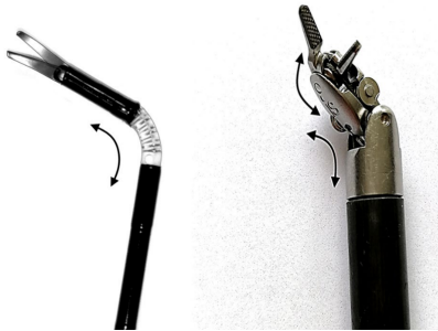
Figure 2-3: Examples of cable driven steering mechanisms. Left: backbone based articulation. Right: articulation by conventional hinges (Figure copied from [20]).
