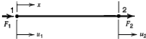
Figure 4-3 Bar under axial forces
