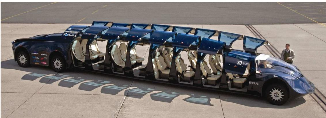
**Figure 1.1:** Superbus side view with opened top hinging doors. Due to the aerodynamic shape of the vehicle, Superbus' appearance greatly differs from traditional buses seen in dense urban areas.
