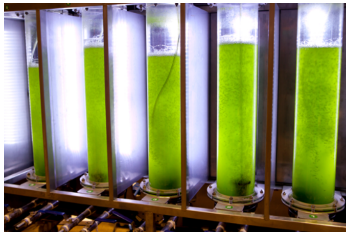
Figure 2.1: Bioreactors contains with live algae cells. Source: Aerin Einstein-Curtis [22].
